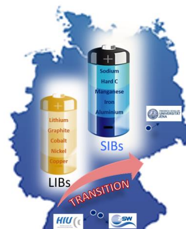
A German consortium will cooperate together to realize powerful liquid and polymeric sodium-ion batteries for electro-mobility and stationary energy storage application (Graphic: Ivana Hasa, KIT)
